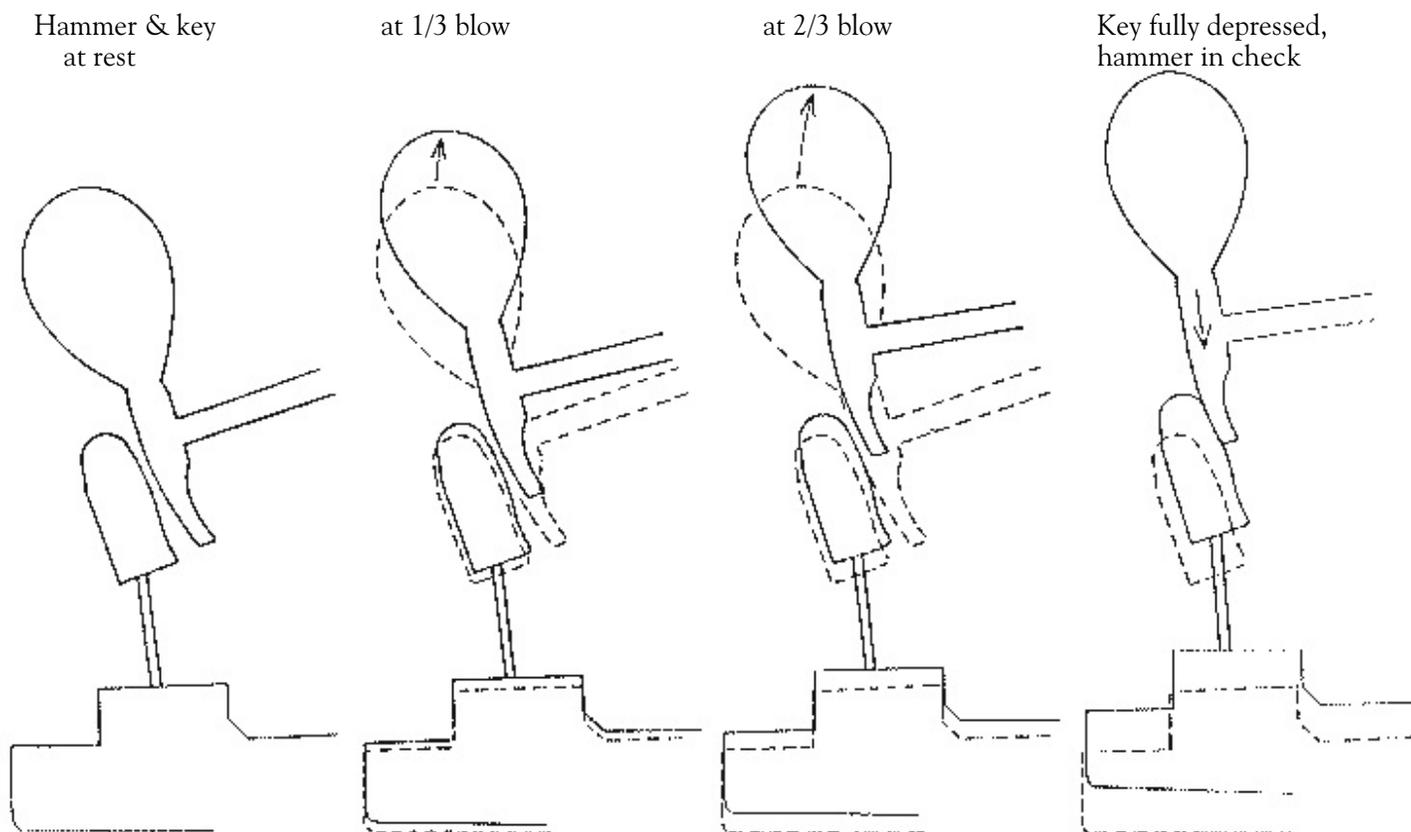
*Note that the tail and backcheck pass with even clearance, and wedge tightly together with good contact area when in check*
